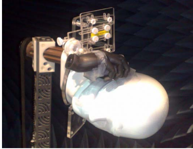
IXBH-060 fixture with PDA hand on ETS MAPS
