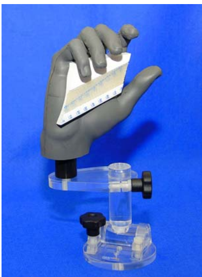
Fixtures shown with IndexSAR standard hands L & R and IXB-090R
