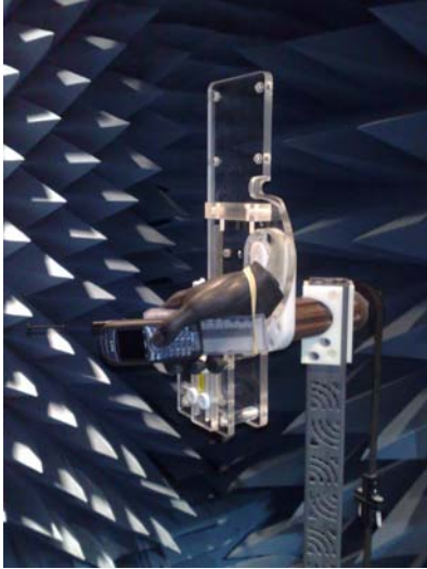
Data hand free space fixture on ETS-Lindgren 'MAPS' OTA system
